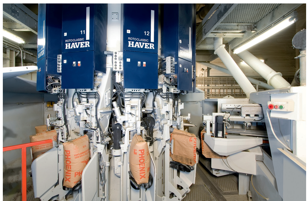
A Haver & Boecker classic: for over 50 years the HAVER ROTO-PACKER® has been deployed for material filling.
